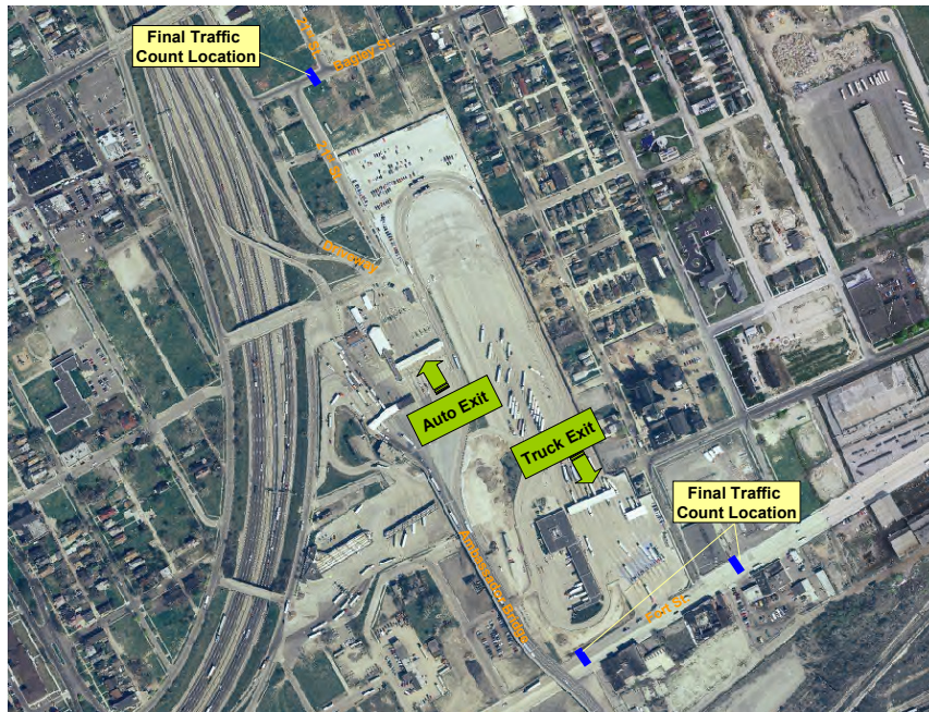
Figure 3-13. Traffic Count Locations at the US side for the Traffic Entering US through the Ambassador Bridge
